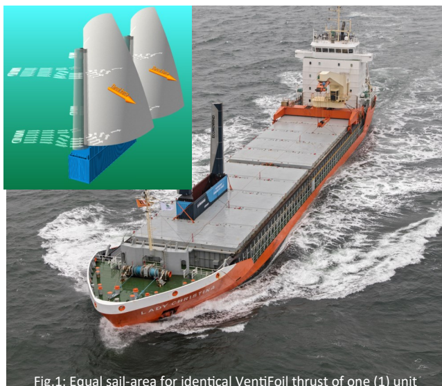
Fig.1: Equal sail-area for identical VentiFoil thrust of one (1) unit
