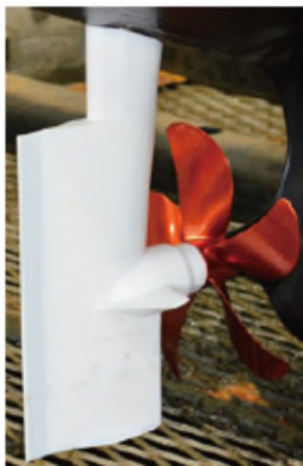
Fig. 2. Model of the energy-saving rudder with bulb fins
